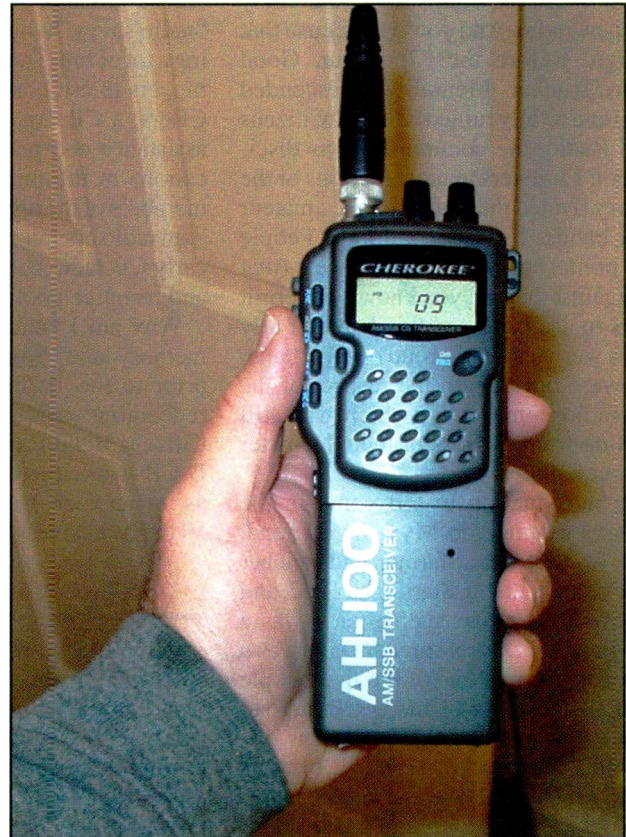
This handheld Cherokee AH-100 is a full-featured AM/SSB 40-channel CB with instant Channel 9 access. It's a great walkie-talkie, but if you don't need all the bells and whistles you'll spend a lot less for instant Citizens Band communications.
