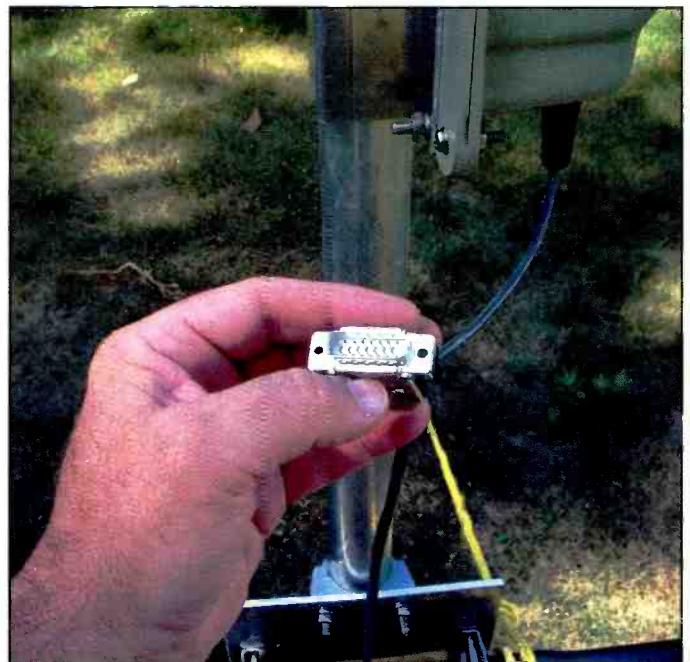
The 15-pin male connector gets filled with silicone grease (included), then plugs into the included wiring harness, which then plugs into the antenna.
