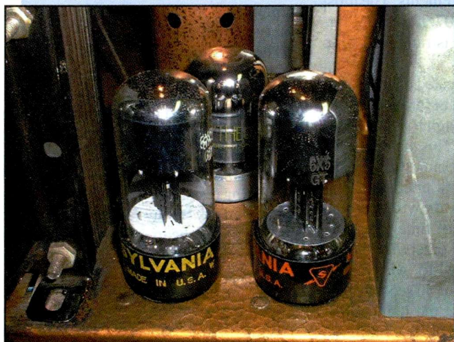
Photo C. The 6X5GT rectifiers are in a prominent spot on the rear chassis, so keeping them glowing is important to the esthetics of the restoration. They are still doing their job, and the likelihood of damage due to rectifier failure has been greatly diminished.
